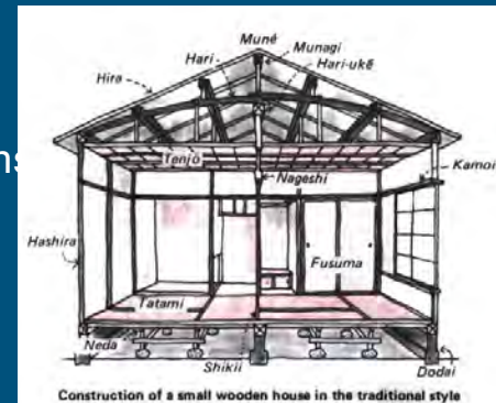
Construction of a small wooden house in the traditional style
